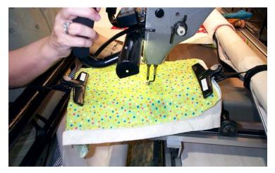
Testing your machine's tension has never been easier! You can wrap the Grip-Lite clamp's double-sided Velcro strip to create a short grip on a piece of test fabric and batting. No need to test on the actual quilt itself or take a chance by not calibrating the tension first.
